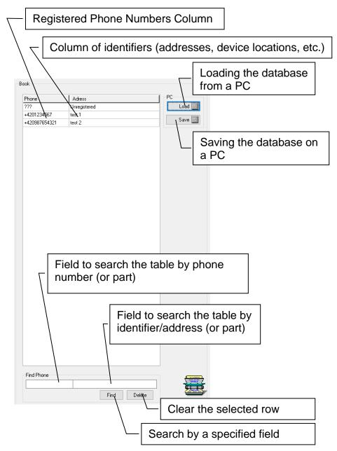
• The database of registered numbers is loaded automatically when the program is started (if it has a name CallMonitor.csv) or by pressing the "Load" button.
