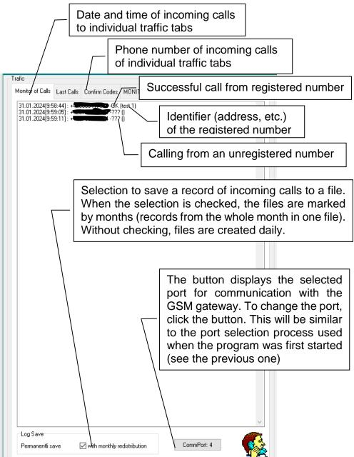
During an incoming registered call, a row with the relevant registration is automatically selected and displayed in the registered numbers database table for better identification.
