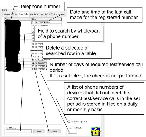
The table shows a list of registered phone numbers with the date and time of the last recorded call. It is functional only in the program mode for handling test/service calls (for periods 1-9). The program scans the table every midnight and creates a list of numbers where the time from the call to the current date is greater than the set period. Lists can be saved by days or months according to requirements (as well as the length of the device list).
