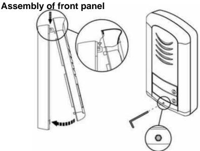
**CAUTION!** During assembly of front panel you might connect/disconnect speaker connector (via schematics)
