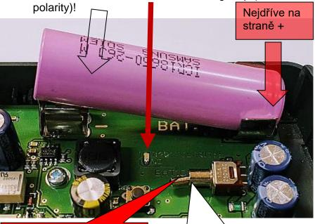
Before inserting the battery, turn off the battery by sliding the switch lever to the position away from the battery holder.
