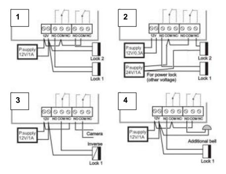
**CAUTION!** Relay contacts can't close 230V directly. To control directly 230V devices you must use contactor.
