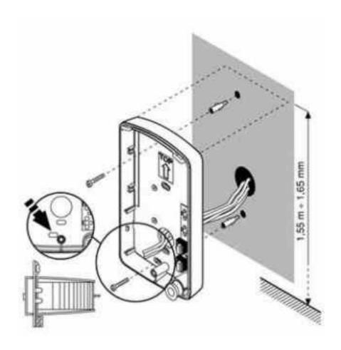
Replacing backlighting cards after wall mounting
