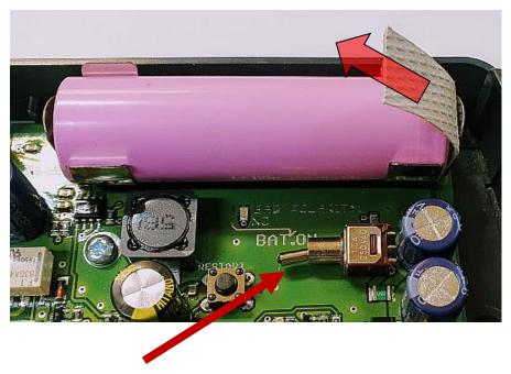
Turn on the battery: move the switch lever to a position closer to the battery holder
