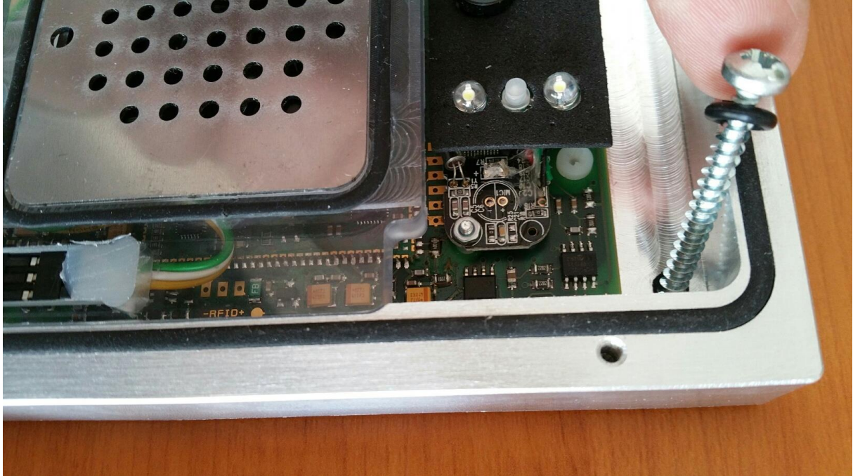
Fig 12. Use screws with rubber rings to avoid any leakages inside the unit
