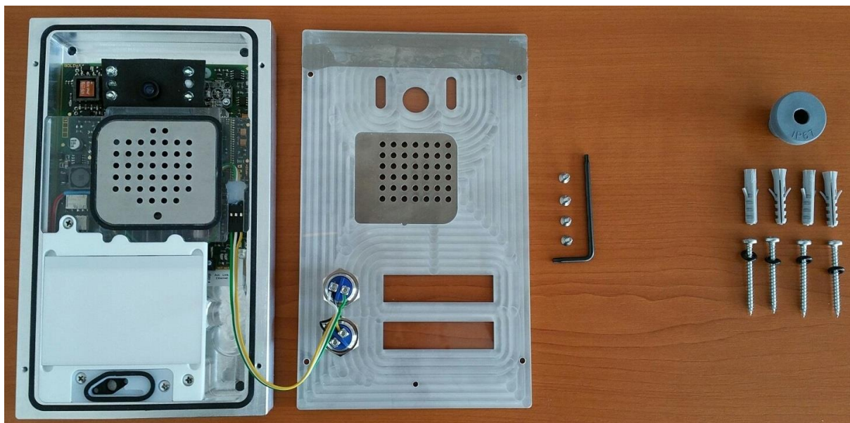
Fig 4 – Open your IP BOLD65 using a supplied allen key, make sure you do not damage the cable connector, connection to the call buttons or the cable itself. It is better to disconnect the call buttons cable.
