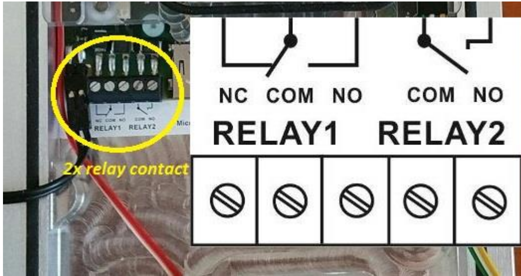
Fig 15 Relay contacts of the IP BOLD65 doorphone
