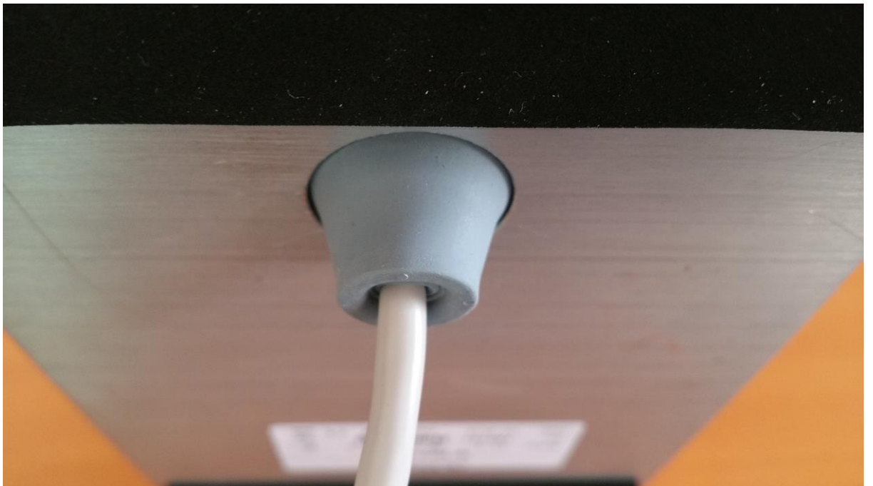
Fig 10. Use the rubber busing with IP67 impregnation rating to avoid any leakages inside the unit. Make sure there is enough space behind the unit inside the wall to avoid jamming the cables, damaging the rubber busing and damaging the cables.
