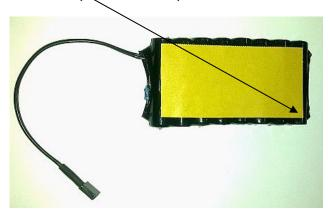
3. Glue the akupack to the lid of the box. WARNING about the holes for the signaling LED! DON'T COVER UP!
