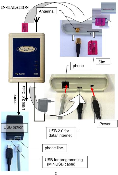
Insert the SIM card oriented as shown on the previous page and press to secure it in the working position. We recommend that you check its status on any GSM phone before inserting the SIM card (switching on with PIN, or without PIN, PIN, etc.) and set them on without PIN. If you want to use PIN on, you must set this PIN when programming the gateway (see programming table). Without this setting, the gateway will not be in operation!
